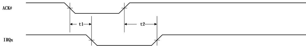
**Table 9-15. Control Signal Delay Time of Parallel Port Timing**
