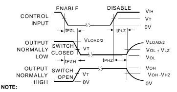
Diagram shown for Input Control Enable-LOW and Input Control Disable-HIGH.
