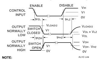
Diagram shown for input Control Enable-LOW and input Control Disable-HIGH.
