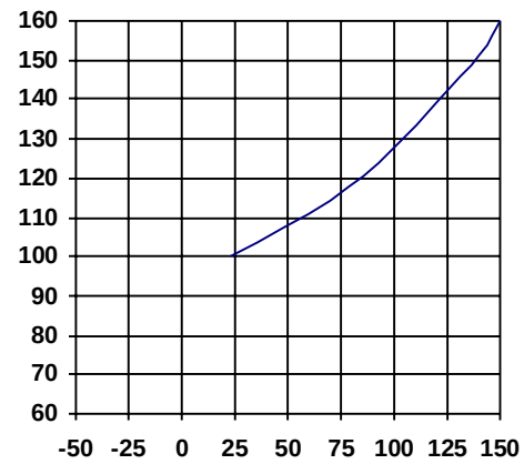
Figure 6 - Normalised R_{ds(on)} (%) Vs T_j (°C)
