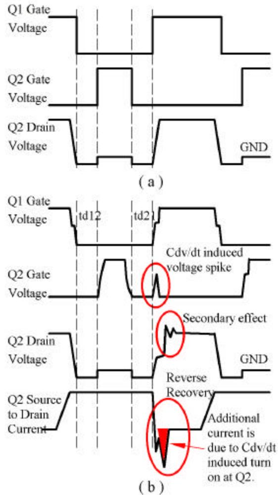
**Figure 2.** (a) Ideal waveforms in a synchronous buck voltage regulator; (b) waveforms due to Cdv/dt induced turn-on at Q2.
