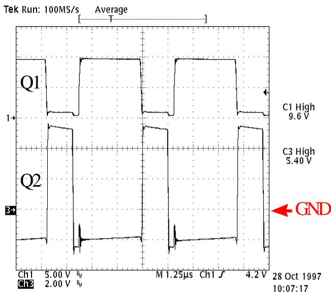
Figure 10. AC gate drive waveforms.
