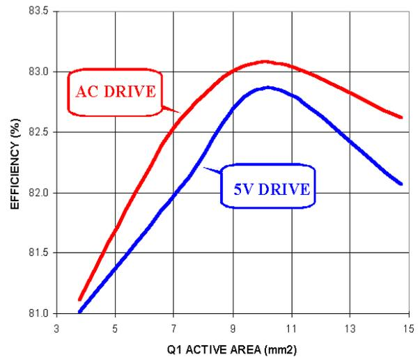
Figure 11. Measured efficiency on ac and 5V dc drives.
