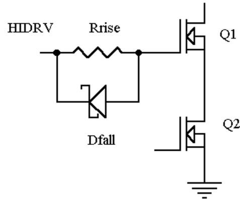
Figure 8. Asymmetric gate drive for MOSFET Q1.
