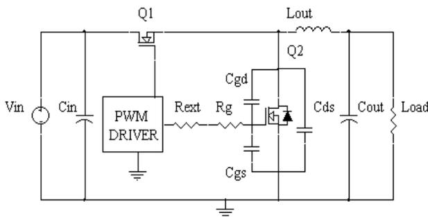
Figure 4. Detailed representation of Q2 in a synchronous buck regulator.
