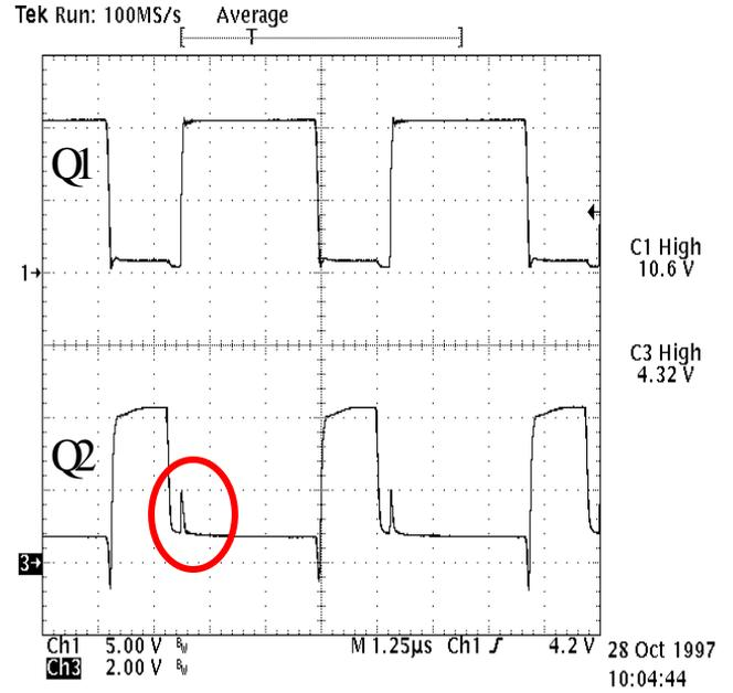
Figure 7. Cdv/dt effect on the gate voltages.
