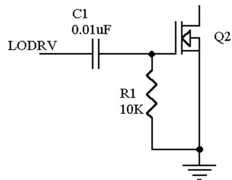
Figure 9. AC gate drive for MOSFET Q2.
