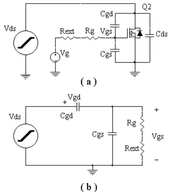
Figure 5. (a)  $C_{dv}/dt$  induced turn-on model circuit. (b) Equivalent circuit of (a).
