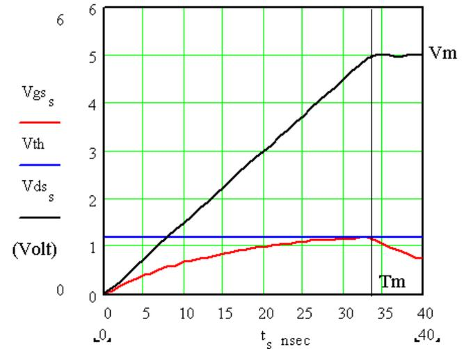
Figure 6. Minimum  $dv/dt$  to cause  $V_{gs} \geq V_{th}$ .
