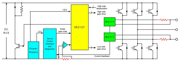
The chipset user can choose between its built-in, optional space vector pulse width modulator (SVPWM) or an external modulation technique. Programming of the modulator can be accomplished through different input coordinates introduced through a serial interface:
