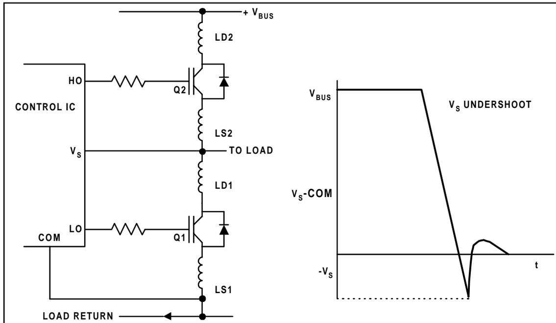
Figure 1. Parasitic Elements of the Half Bridge
