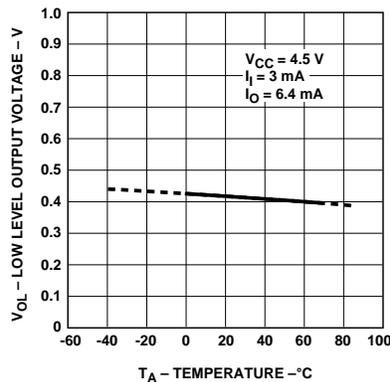
**Figure 6. Typical Logic Low Output Voltage vs. Temperature.**
