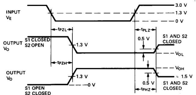
Figure 13. Waveforms for  $t_{PZH}$ ,  $t_{PZL}$ ,  $t_{PHZ}$ , and  $t_{PLZ}$ .
