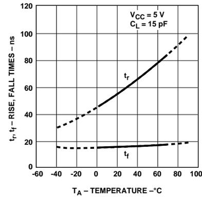
Figure 11. Typical Rise, Fall Time vs. Temperature.
