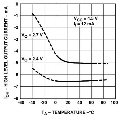
**Figure 7. Typical Logic High Output Current vs. Temperature.**
