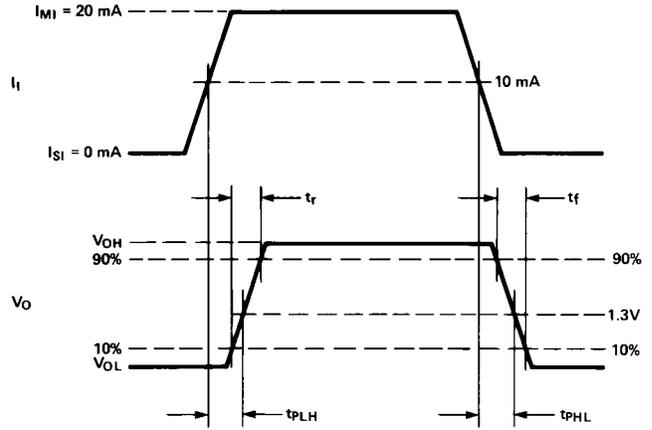
Figure 9. Waveforms for  $t_{PHL}$ ,  $t_{PLH}$ ,  $t_r$ , and  $t_f$ .
