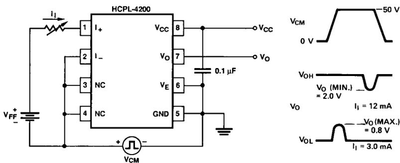
Figure 16. Test Circuit for Common Mode Transient Immunity.
