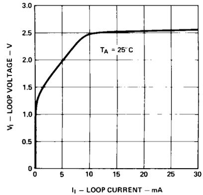
**Figure 4. Typical Input Loop Voltage vs. Input Current.**
