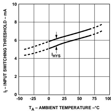
**Figure 3. Typical Current Switching Threshold vs. Temperature.**
