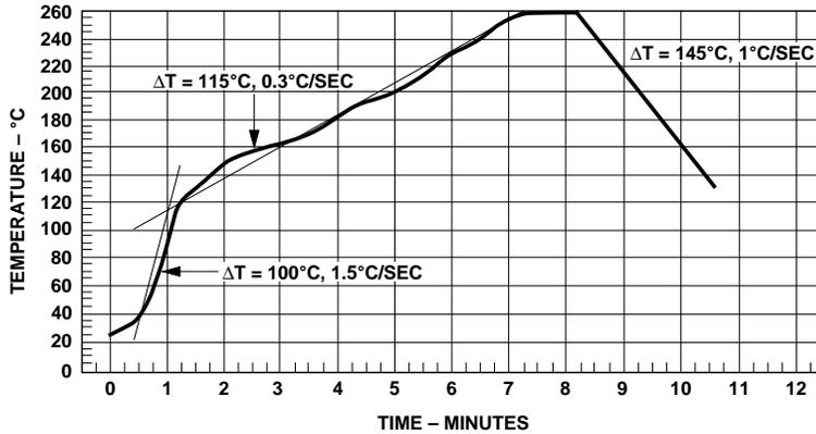
Figure 1. Maximum Solder Reflow Thermal Profile.
