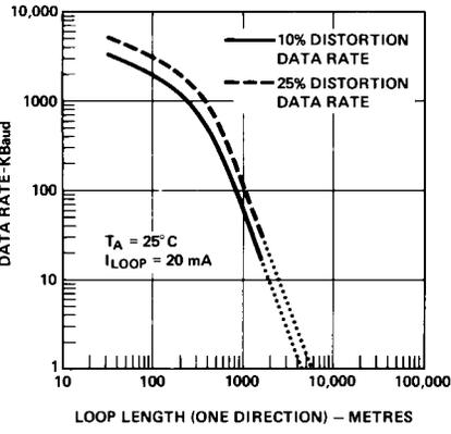
**Figure 20. Typical Data Rate vs. Distance.**
