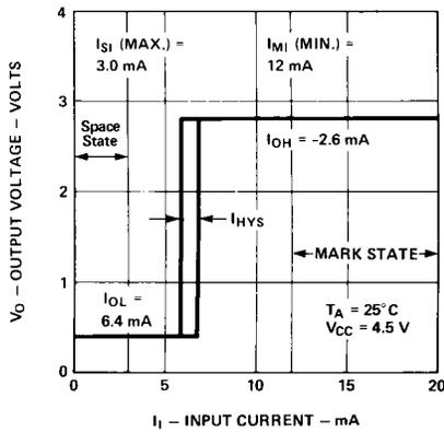
**Figure 2. Typical Output Voltage vs. Loop Current.**
