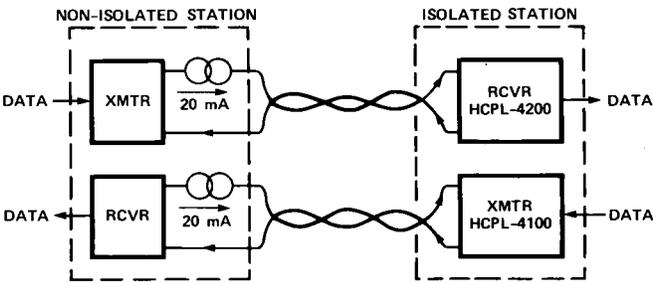
**Figure 21. Full Duplex Point-to-Point Current Loop System Configuration.**
