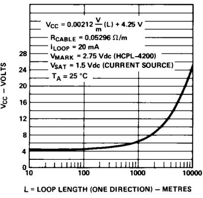
**Figure 19. Minimum Required Supply Voltage, V<sub>CC</sub>, vs. Loop Length for Current Loop Circuit of Figure 19.**
