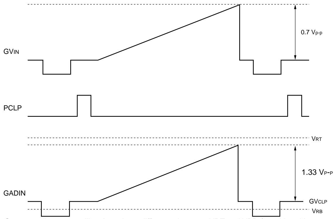
Contrast adjust : controlling the voltage difference between  $V_{\text{RT}}$  and  $V_{\text{RB}}$  (typ :  $V_{\text{RT}} - V_{\text{RB}} = 1.33 \text{ V}$ )
