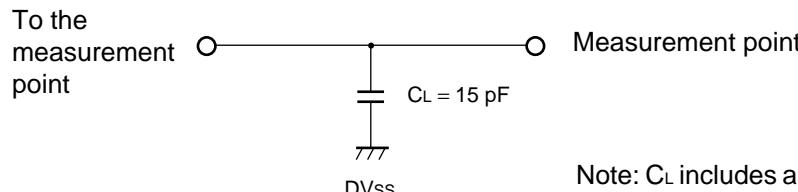
Note: CL includes a stray capacitance of a probe and a fixture.
