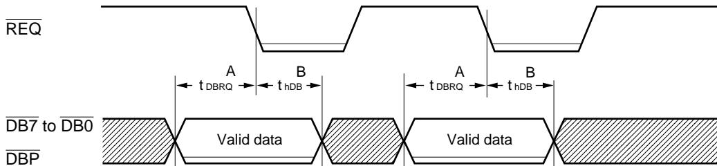
**MB86604L****(8) A/N/S values in the SCSI interface timing specification**
