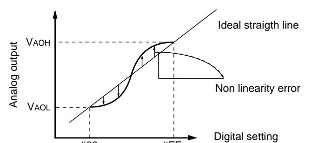
Note : The value of  $V_{AOH}$  and  $V_{DD}$ , and the value of  $V_{AOL}$  and  $V_{SS}$  are not necessarily equivalent.
