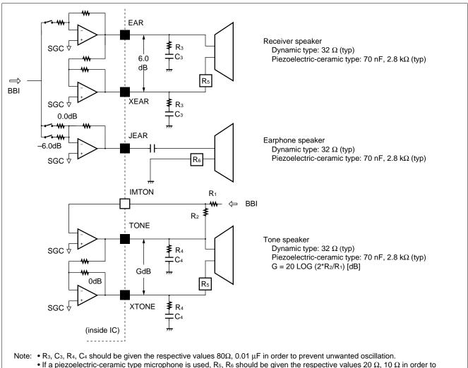
If a piezoelectric-ceramic type microphone is used, R<sub>5</sub>, R<sub>6</sub> should be given the respective values 20 Ω, 10 Ω in order to
