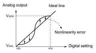
Note:The value of VaoH and Vdd, and the value of VaoL and GND are not necessarily equivalent.
