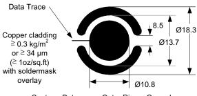
Center – Data Outer Ring – Ground All dimensions are in millimeters.
