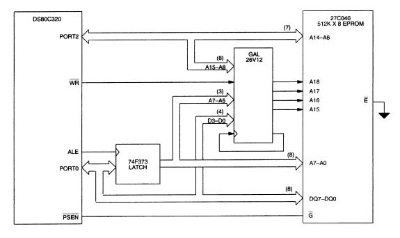
The following software example shows an assembly language routine to jump to a new location in any bank using latched data as shown in Figure 6. Before calling the bank switch subroutine, software pushes the new address and bank number onto the stack. It then calls a subroutine that pops the new bank address
