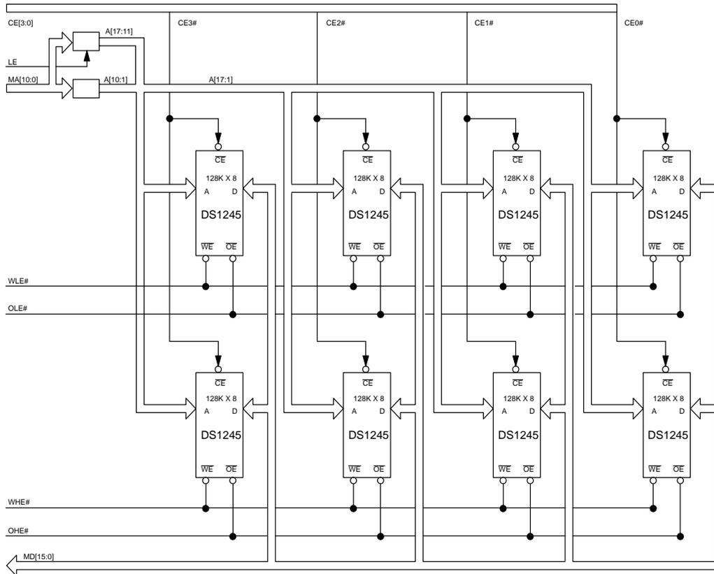
In Figure 6, eight DS1245 SRAMs are used to create a four-bank 1Mbyte SRAM memory subsystem. The following signals from the Intel 386SL CPU are required to address the SRAM module based system. (The 386SL memory controller must be configured in its SRAM addressing mode for this application.)
