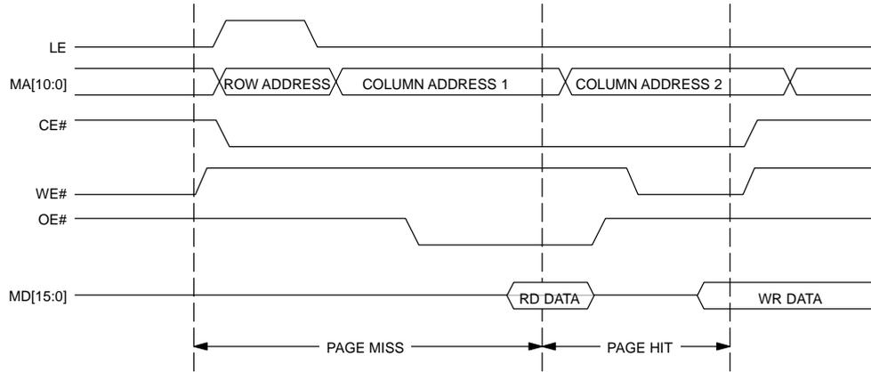
**1 MBYTE MEMORY SUBSYSTEM USING NV SRAMS Figure 6**
