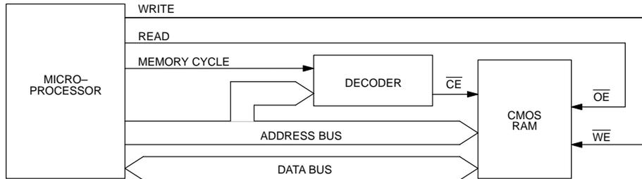
BYTEWISE MEMORIES PROVIDE EASY INTERFACE TO MICROPROCESSORS BECAUSE OF THE X8 ORGANIZATION AND CONTROL SIGNAL DEFINITION.
