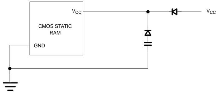
CMOS STATIC RAM REQUIRES MORE THAN JUST A BACKUP POWER SUPPLY. DATA MUST ALSO BE PROTECTED DURING POWER TRANSIENTS TO AVOID GARBLED DATA.
