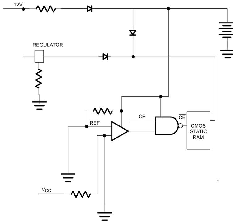
SUPPORT CIRCUITRY REQUIRED TO PRODUCE POWER FAIL DETECTION AND WRITE PROTECTION FORCES THE NEED FOR MULTICELL RECHARGEABLE BATTERY OR A LITHIUM BATTERY.
