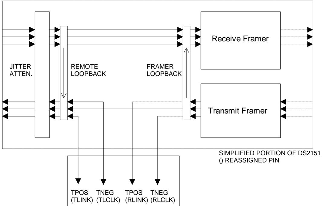
MODE 3: DS2151 Special Mode to Tap the Transmit & Receive Bipolar Data Streams
