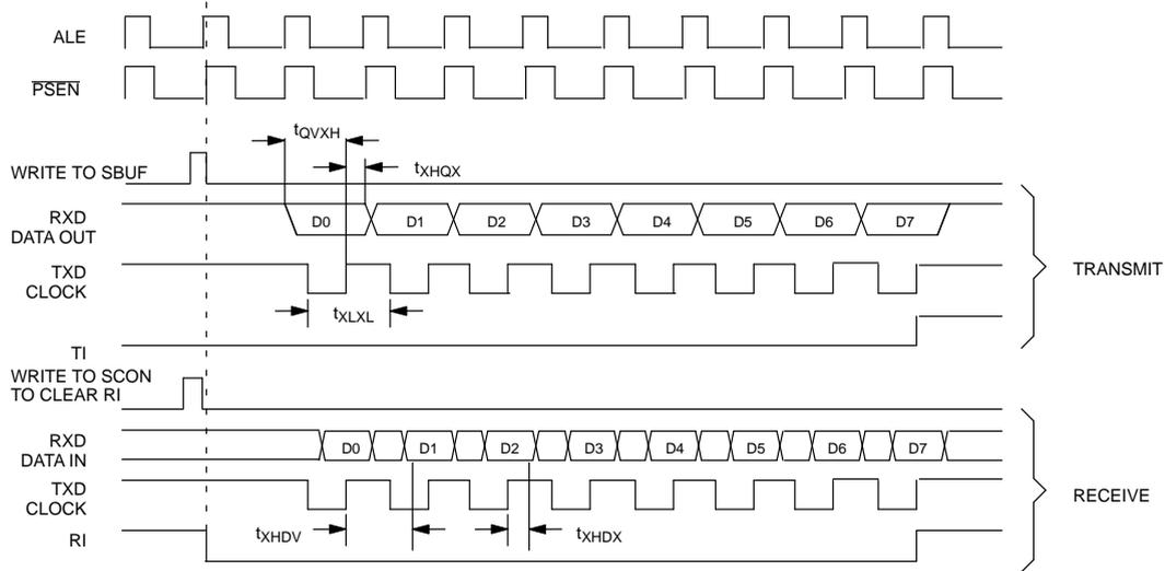
SERIAL PORT 0 (SYNCHRONOUS MODE)
