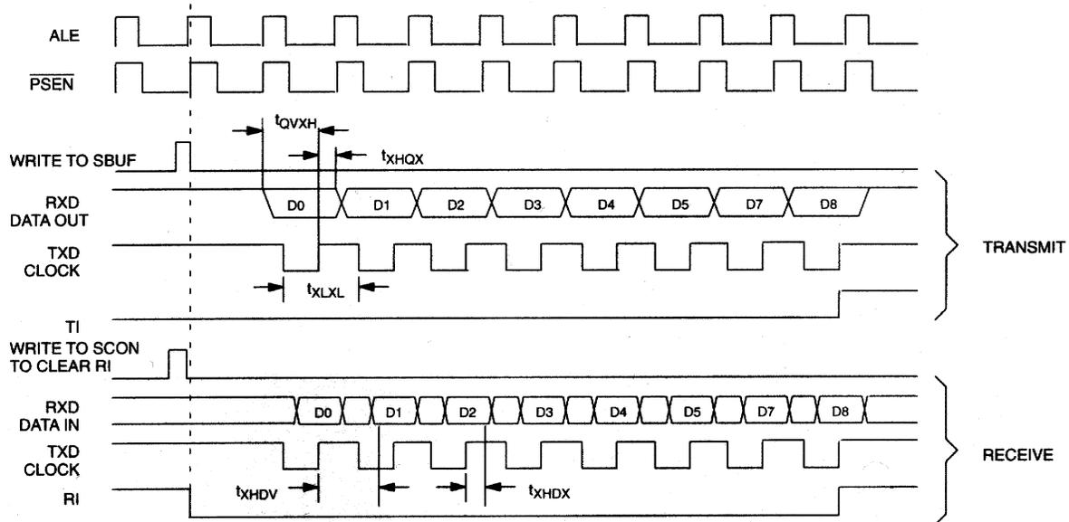
SERIAL PORT 0 (SYNCHRONOUS MODE)
