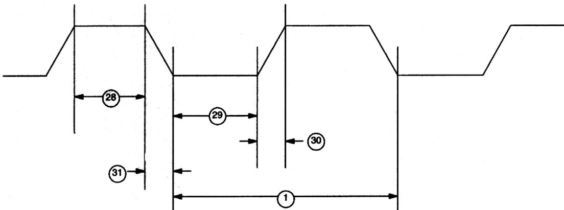
**AC CHARACTERISTICS (cont'd)****POWER CYCLE TIME** $(T_A = 0^\circ\text{C to } 70^\circ\text{C}; V_{CC} = 5V \pm 10\%)$
