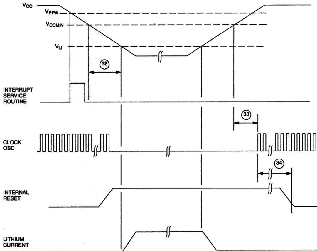
**AC CHARACTERISTICS (cont'd)****SERIAL PORT TIMING - MODE 0** $(T_A = 0^\circ\text{C to } 70^\circ\text{C}; V_{CC} = 5\text{V} \pm 10\%)$
