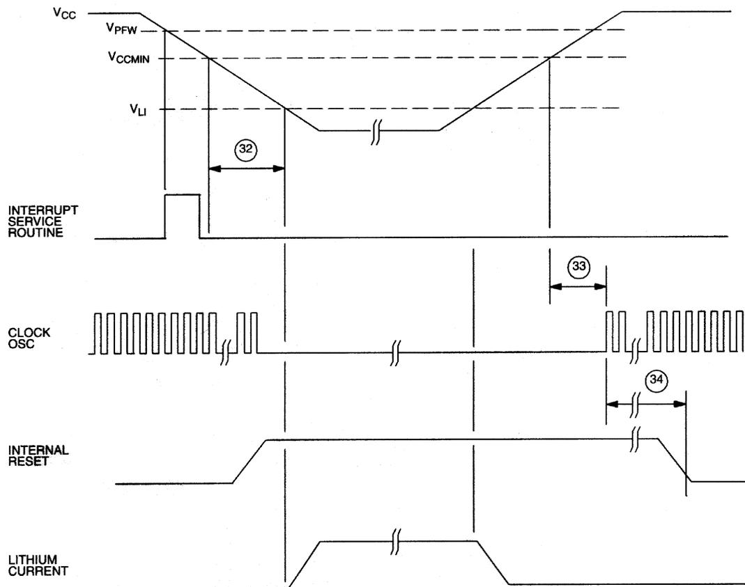
**AC CHARACTERISTICS (cont'd)****PARALLEL PROGRAM LOAD TIMING** $(t_A=0^{\circ}\text{C to }70^{\circ}\text{C}; V_{CC}=5\text{V} \pm 5\%)$
