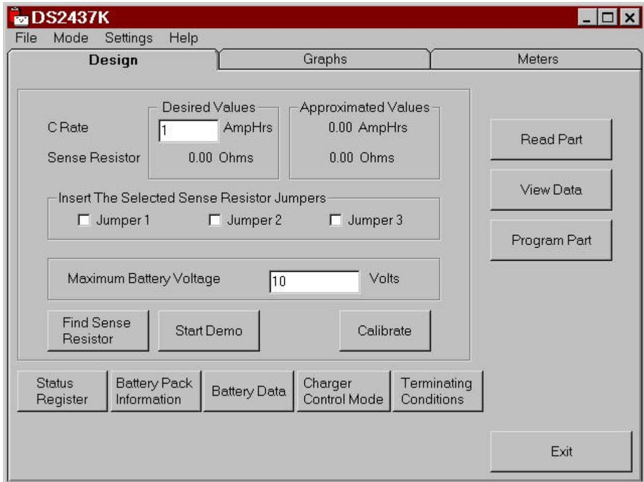
The main difference between the Demo and Design modes is that the Design Mode includes features to set the values of various data fields, program the DS2437 with these values, and read the data back from the DS2437. The Design Screen includes the Read Part, View Data and Program Part buttons on the right side of the screen as well as a number of buttons across the bottom of the screen, each of which pops up a separate data entry window.
