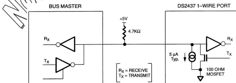
The idle state for the 1-Wire bus is high. If for any reason a transaction needs to be suspended, the bus **MUST** be left in the idle state if the transaction is to resume. Infinite recovery time can occur between bits so long as the 1-Wire bus is in the inactive (high) state during the recovery period. If this does not occur and the bus is left low for more than 480  $\mu$ s, all components on the bus will be reset.
