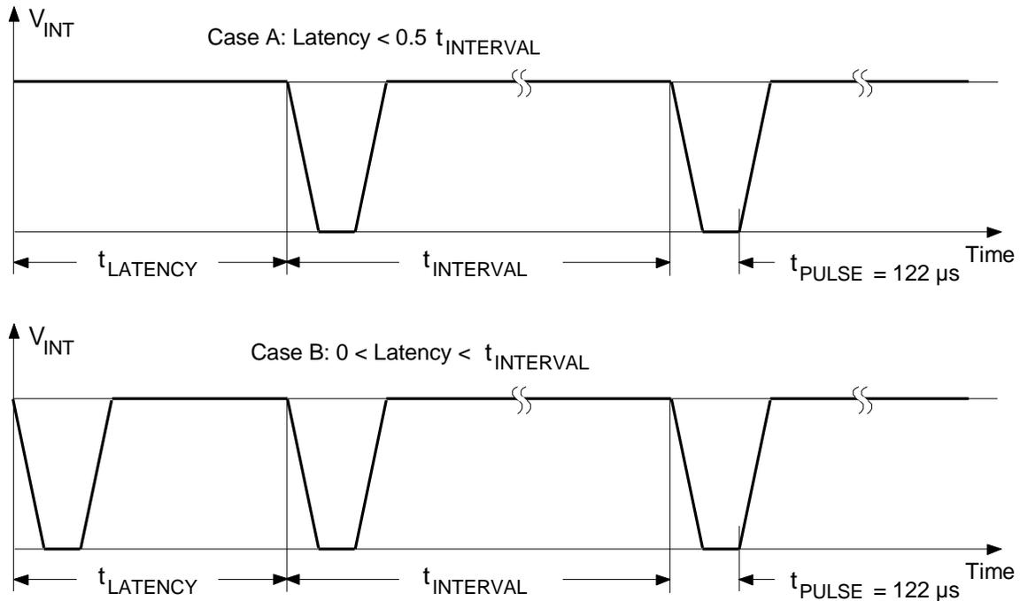
The latency depends on the selected interrupt interval (IS0 to IS2 settings) and the contents of the RTC counter at the time of writing the device control byte. In Case A, the flip-flop that determines the interval duration is reset and toggles before half of the interval time is over. In Case B, this flip-flop is set which generates an immediate interrupt pulse; the latency, therefore, can be up to one full interval duration.
