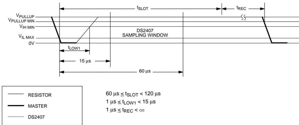
**READ/WRITE TIMING DIAGRAM** Figure 15 (cont'd)**Write-zero Time Slot**
