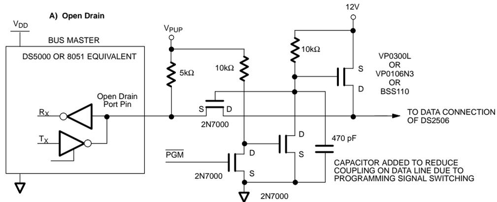
The interface is reduced to the 5kΩ pull-up resistor if one does not intend to program the EPROM cells.
