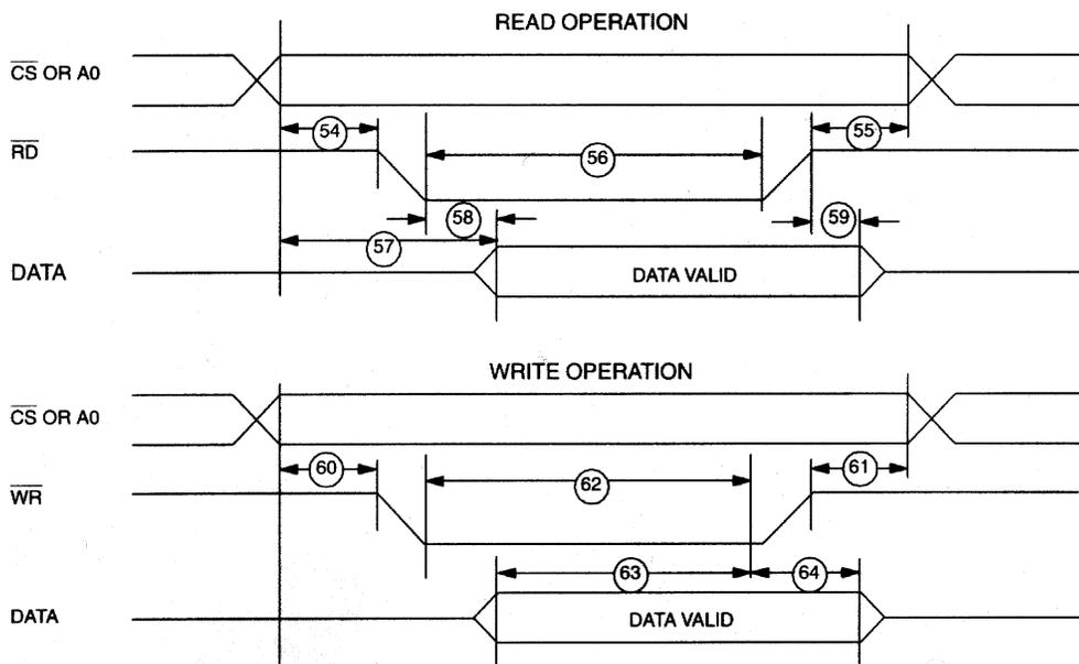
**AC CHARACTERISTICS -  $\overline{\text{PROG}}$**  $(t_A=0^{\circ}\text{C to }70^{\circ}\text{C}; V_{CC}=5\text{V} \pm 10\%)$
