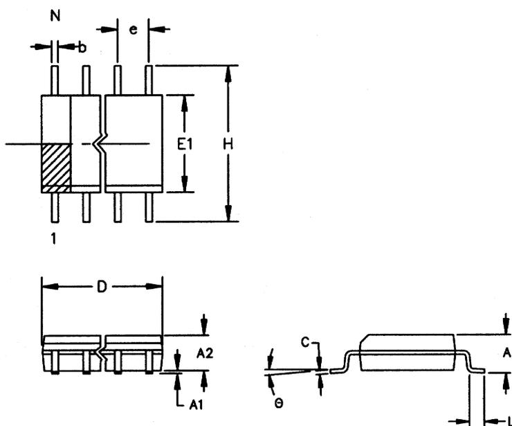
The chamber on the body is optional. If it is not present, a terminal 1 identifier must be positioned so that  $\frac{1}{2}$  or more of its area is contained in the hatched zone.
