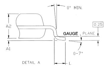
DIMENSIONS ARE IN MILLIMETERS
