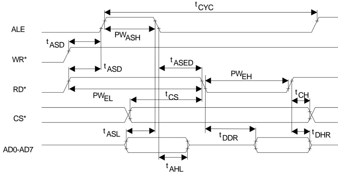
**INTEL BUS WRITE TIMING (BTS=0 / MUX=1) Figure 21-2**
