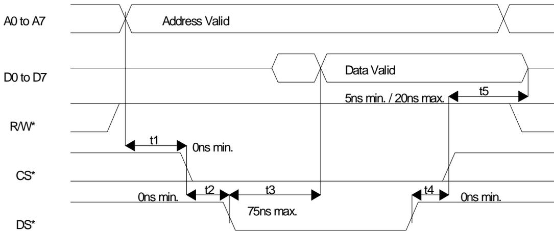
**MOTOROLA BUS WRITE AC TIMING (BTS=1 / MUX=0) Figure 21-7**
