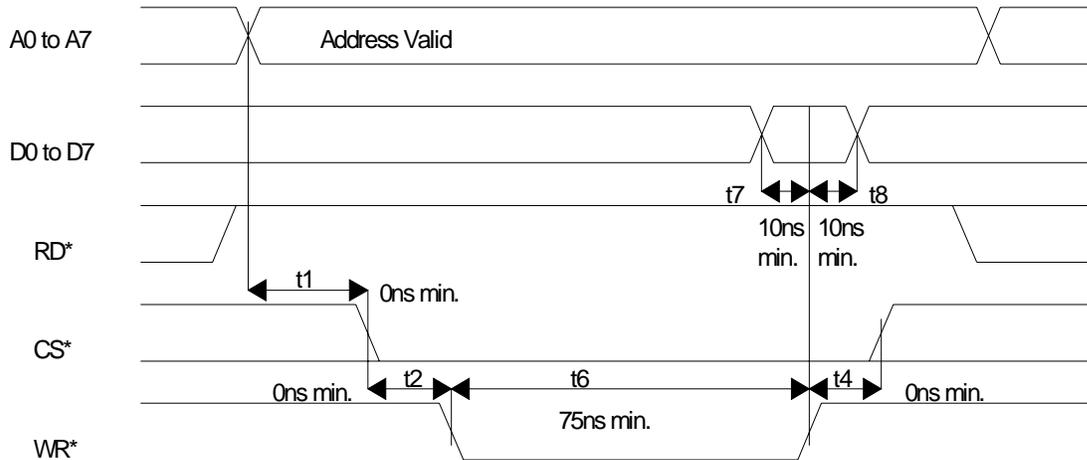
**MOTOROLA BUS READ AC TIMING (BTS=1 / MUX=0) Figure 21-6**
