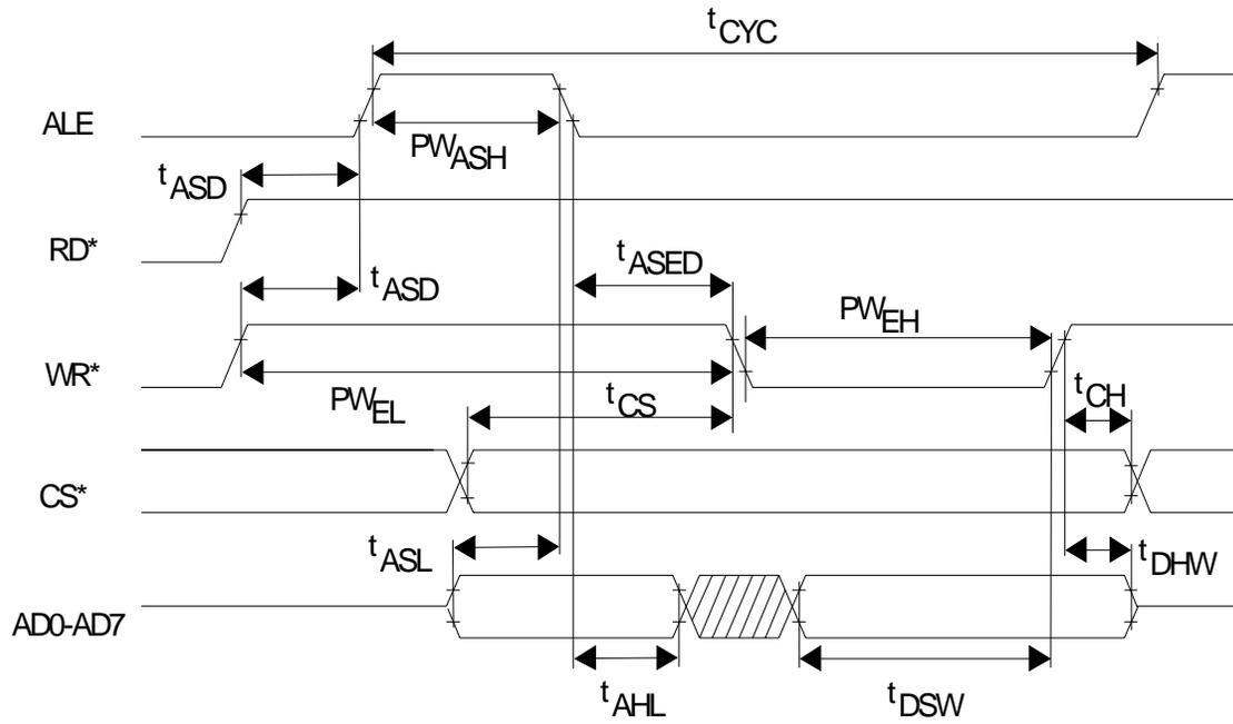
**MOTOROLA BUS AC TIMING (BTS = 1 / MUX = 1) Figure 21-3**
