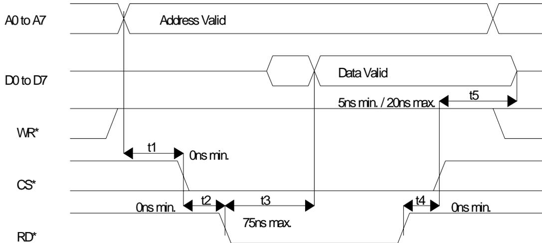
**INTEL BUS WRITE AC TIMING (BTS=0 / MUX=0) Figure 21-5**
