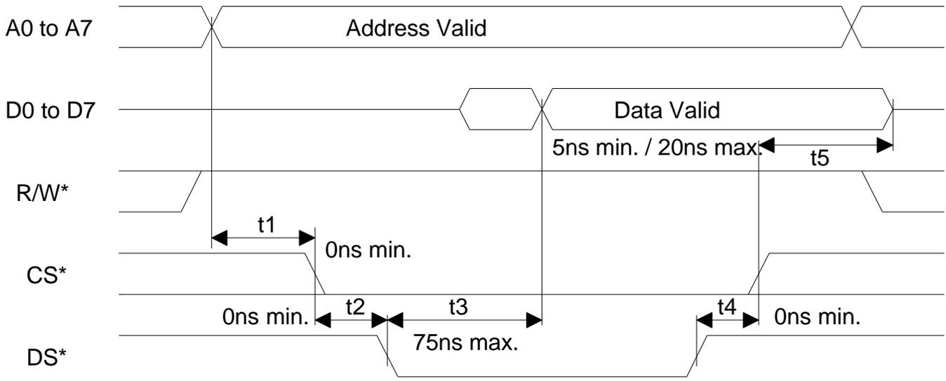
**Figure 24-7 MOTOROLA BUS WRITE TIMING (BTS=1 / MUX=0)**
