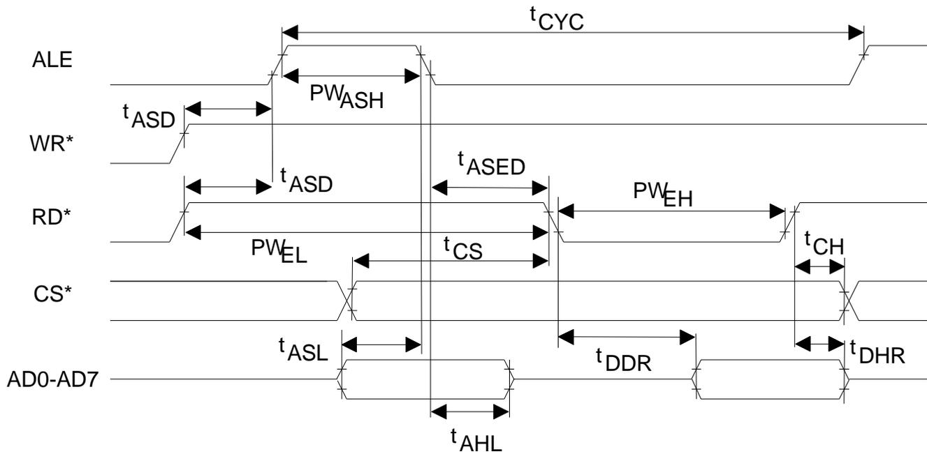
**Figure 24-2 INTEL BUS WRITE TIMING (BTS=0 / MUX=1)**
