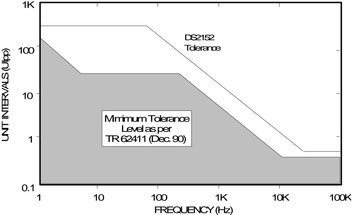
Figure 16-5 JITTER ATTENUATION
