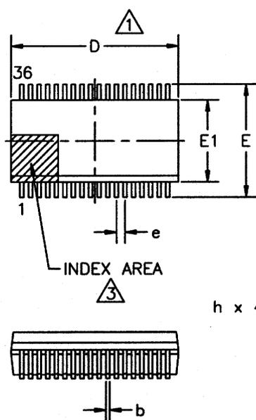
△1 DIMENSIONS D AND E1 INCLUDE MOLD MISMATCH, BUT DO NOT INCLUDE MOLD FLASH, PROTRUSIONS OR GATE BURRS. MOLD FLASH, PROTRUSIONS OR GATE BURRS SHALL NOT EXCEED 0.254 MM PER SIDE.
