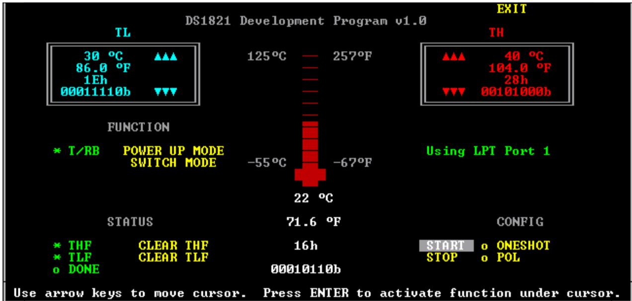
The DS1821K Programmable Digital Thermostat Development Kit allows a potential user of the DS1821 to observe the operation of the DS1821 in an actual temperature measurement application. Temperature is measured and displayed in a text box, as well as on a graphical thermometer.
