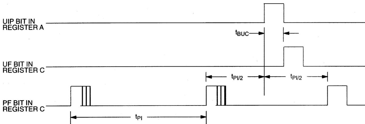
$t_{PI}$  = PERIODIC INTERRUPT TIME INTERNAL PER TABLE 1
