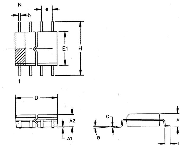
The chamfer on the body is optional. If it is not present, a terminal 1 identifier must be positioned so that ½ or more of its area is contained in the hatched zone.
