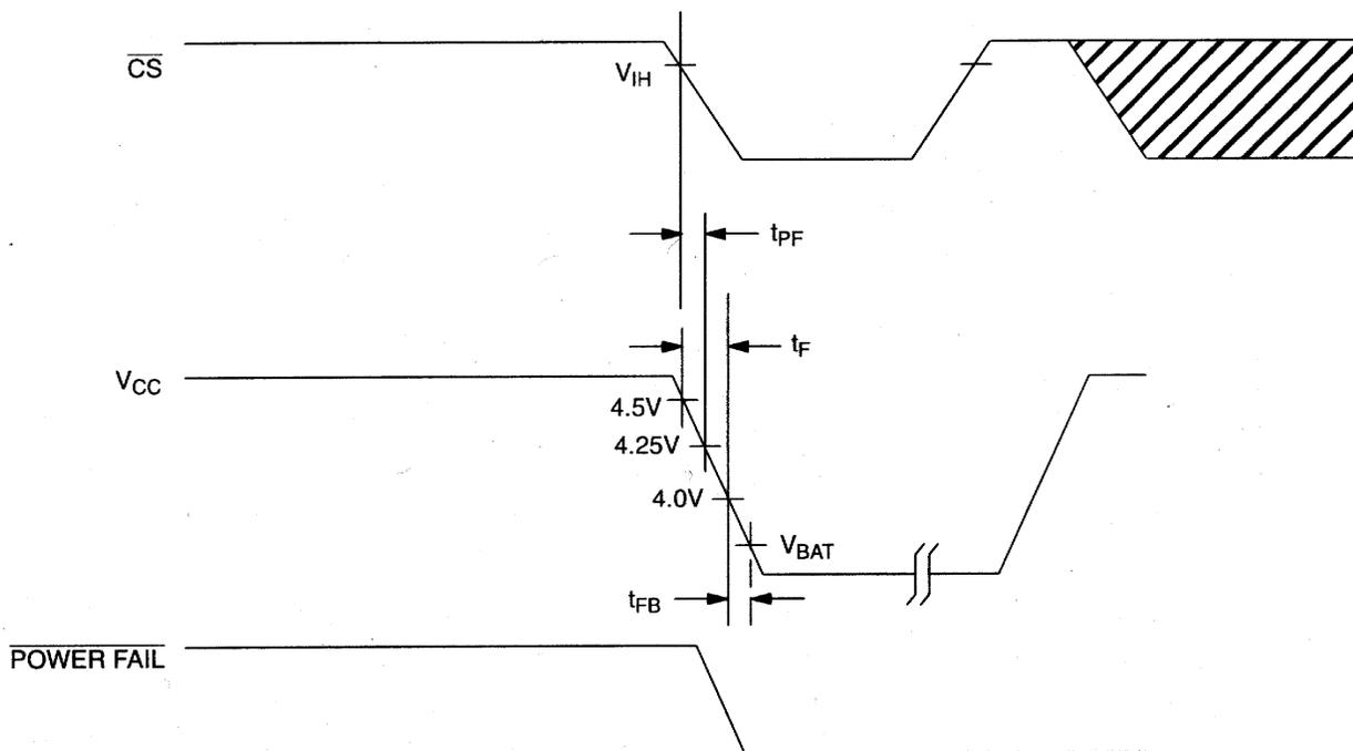
**POWER-UP POWER-DOWN TIMING 5-VOLT DEVICE** (t<sub>A</sub>=25°C)
