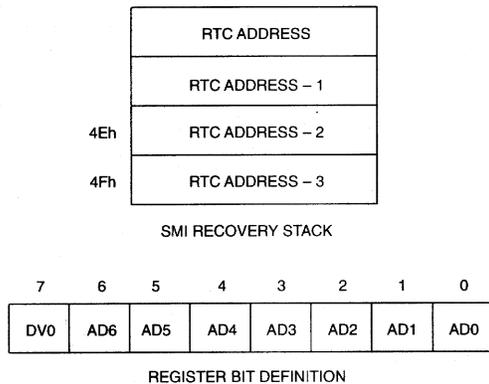
The RTC address is latched on the falling edge of the ALE signal. Each time an RTC address is latched, the register address stack is pushed. The stack is only four registers deep, holding the three previous RTC addresses in addition to the current RTC address being accessed. The following waveform illustrates how the BIOS could recover the RTC address when an SMI occurs.
