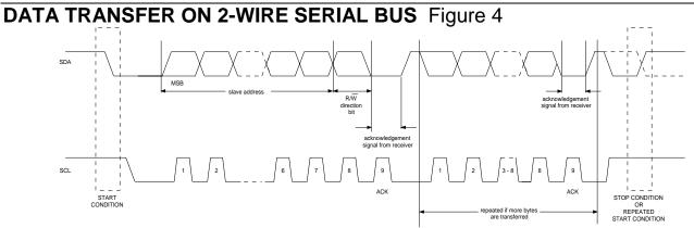
Figures 5 and 6 detail how data transfer is accomplished on the 2-wire bus. Depending upon the state of the  $R/\overline{w}$  bit, two types of data transfer are possible:
