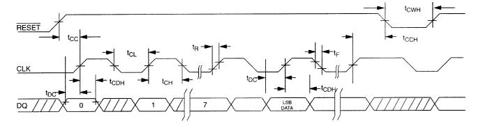
NOTE:  $t_{CL}$ ,  $t_{CH}$ ,  $t_R$ , and  $t_F$  apply to both read and write data transfer.
