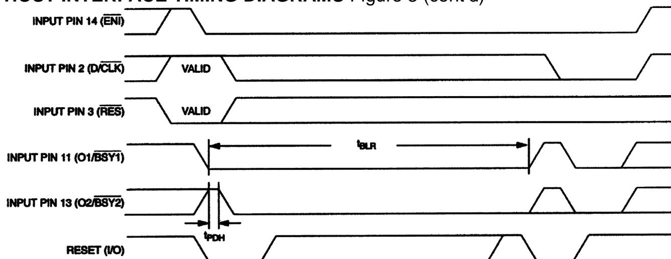
$t_{\text{PDH}} = 2 \mu\text{s}$  (TYPICAL)
