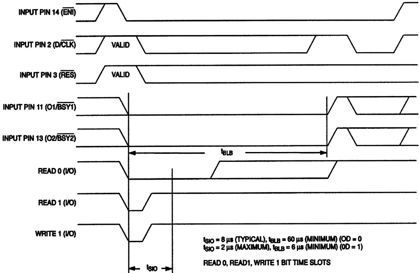
HOST INTERFACE TIMING DIAGRAMS Figure 2 (cont'd)
