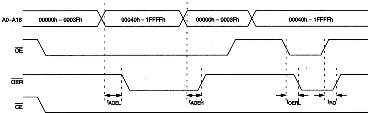
**WRITE CYCLE TIMING: RTC AND EXTERNAL SRAM CONTROL SIGNALS**
