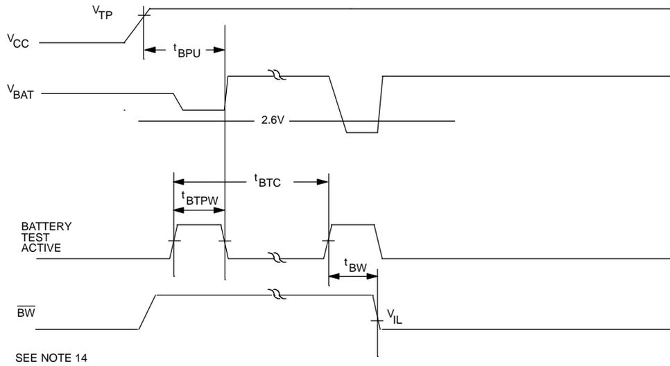
**POWER-DOWN/POWER-UP TIMING**(t<sub>A</sub>: See Note 10)
