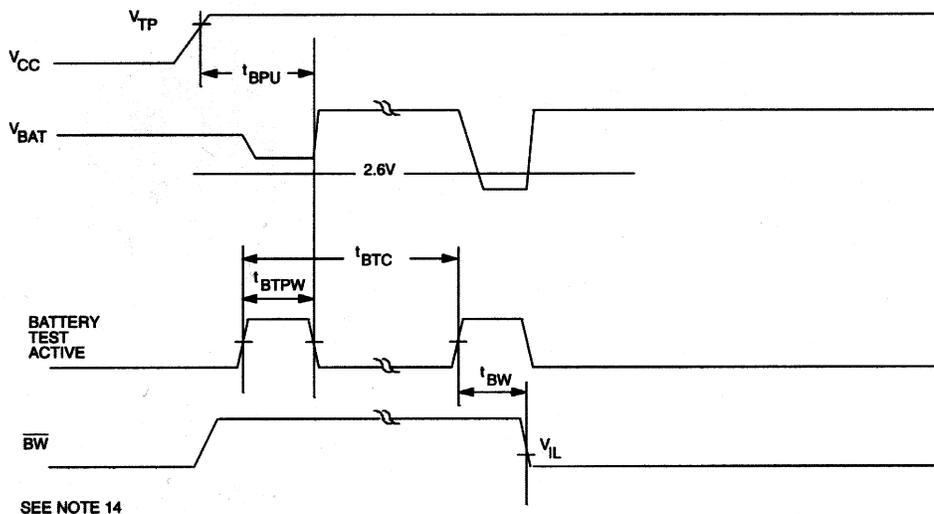
**POWER-DOWN/POWER-UP TIMING**(t<sub>A</sub>: See Note 10)
