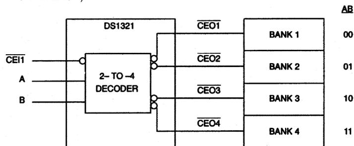
MODE =  $V_{CC0}$  (2 BANKS WITH 2 SRAM EACH):
