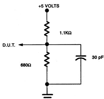
\*INCLUDING SCOPE AND JIG CAPACITANCE
