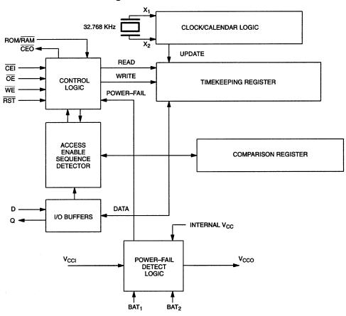
Communication with the Time Chip is established by pattern recognition of a serial bit stream of 64 bits which must be matched by executing 64 consecutive write cycles containing the proper data on data in (D). All accesses which occur prior to recognition of the 64-bit pattern are directed to memory via the chip enable output pin ( $\overline{\text{CEO}}$ ).
