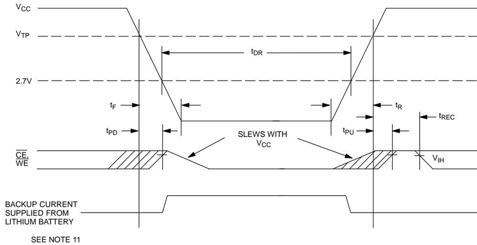
**POWER-DOWN/POWER-UP TIMING**(t<sub>A</sub>: See Note 10)
