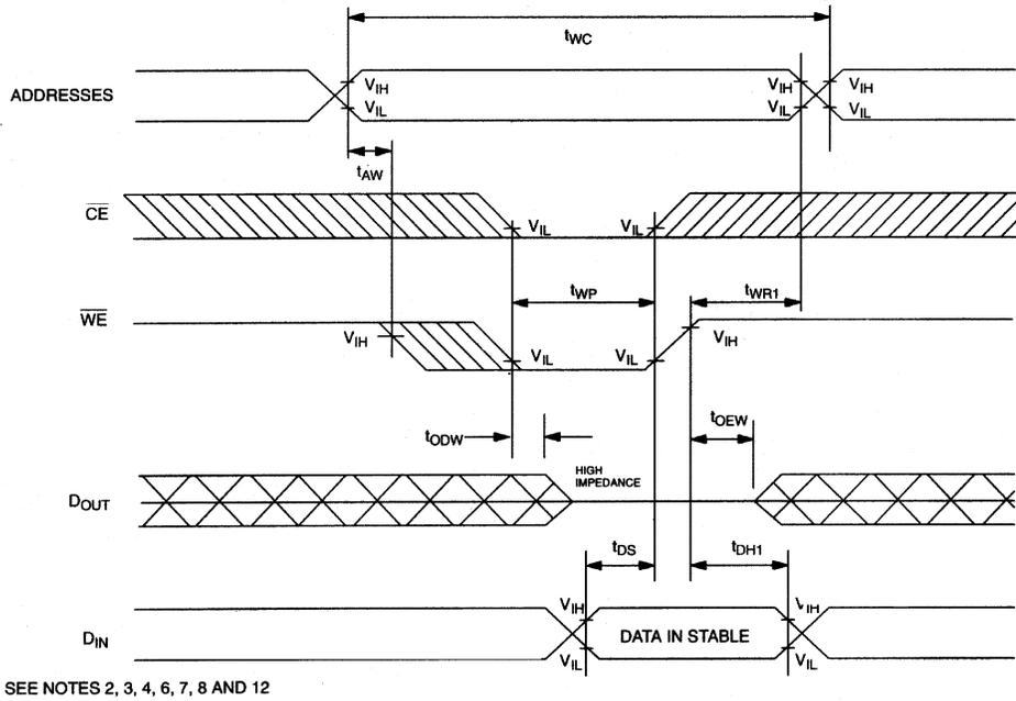
**TIMING DIAGRAM: WRITE CYCLE 2**
