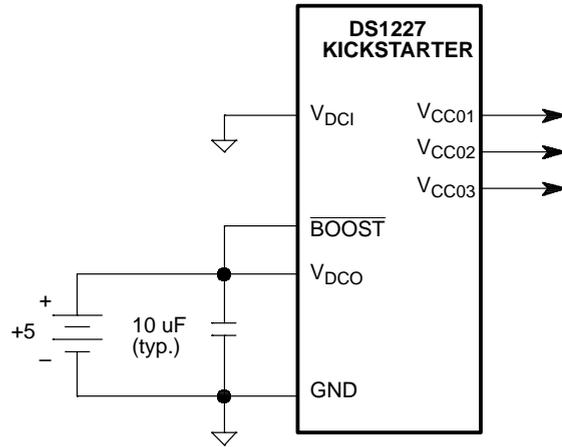
**DS1227 +6V PASS-THROUGH MODE CONFIGURATION** Figure 3
