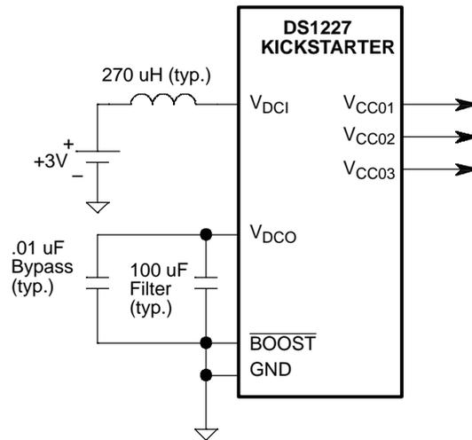
**DS1227 +5V PASS-THROUGH MODE CONFIGURATION** Figure 2
