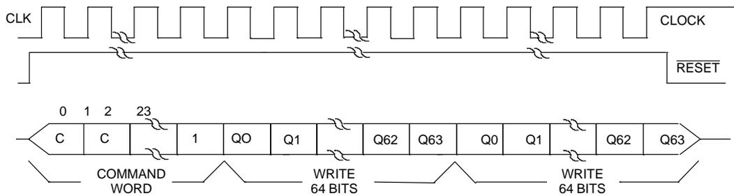
**DATA TRANSFER: PROGRAM MODE, DAY CLOCK, DAYS REMAINING AND OSCILLATOR CONTROL** Figure 15B
