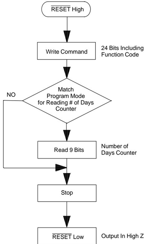
**SEQUENCE: PROGRAM MODE, READING THE 9-BIT NUMBER OF DAYS COUNTER** Figure 6B
