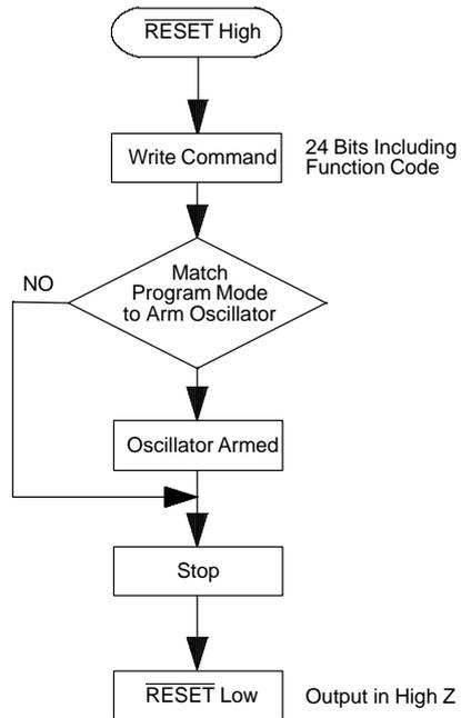
**FLOW CHART: PROGRAM MODE, STOP OSCILLATOR** Figure 10
