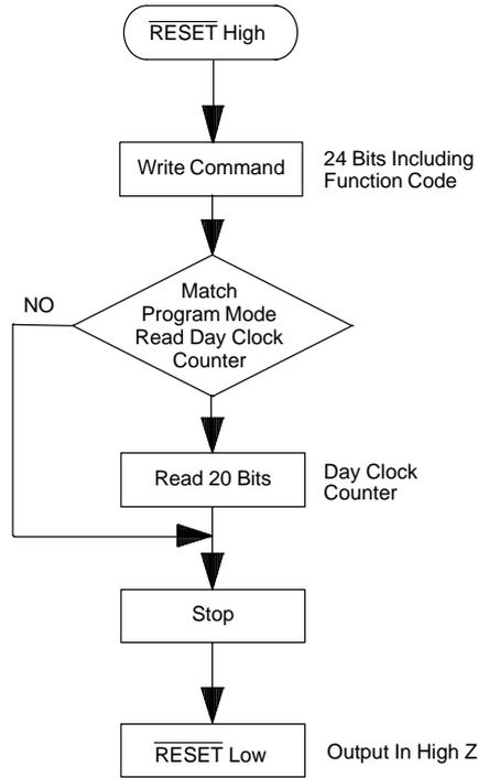
**SEQUENCE: PROGRAM MODE, READING THE 20-BIT DAY CLOCK COUNTER** Figure 5B
