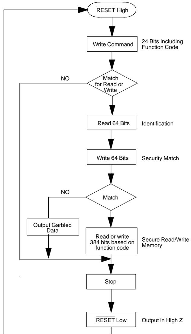
**SEQUENCE: NORMAL MODE, READ OR WRITE SECURE MEMORY** Figure 2B
