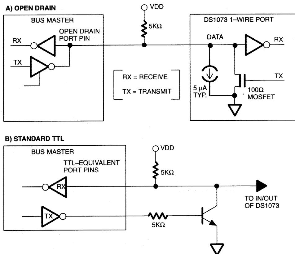
Programming mode is entered by simply powering up the DS1073 with a pullup of approximately  $5k\Omega$ . This will pull the IN/OUT pin above  $V_{IH}$  on power-up and initiate the programming mode, causing the DS1073 to internally release the IN/OUT pin (after  $t_{POR}$ ), and allow the pullup resistor to pull the pin to the supply rail and await the Master Tx Reset pulse (see diagram).
