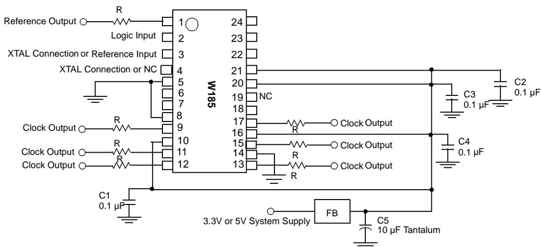
**Figure 4. Recommended Circuit Configuration**
