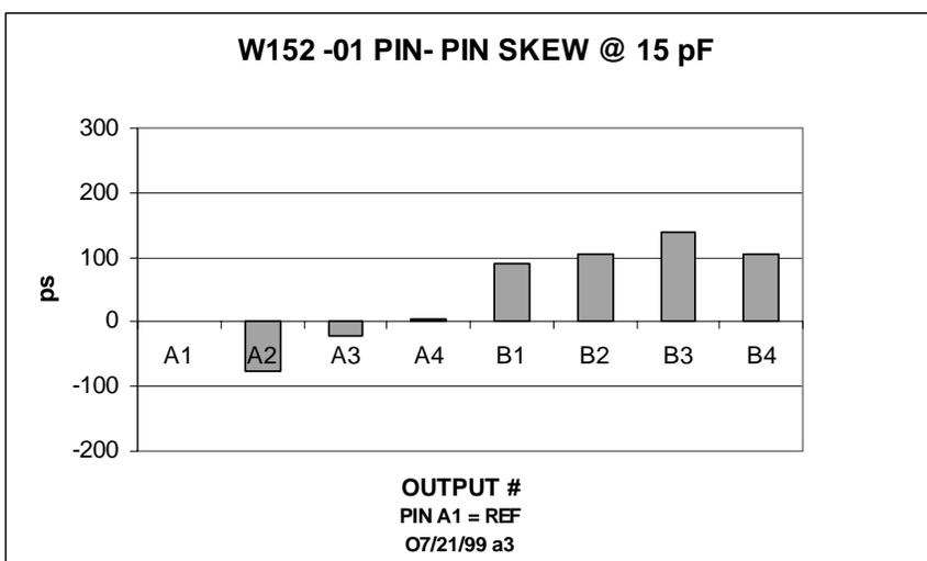
Figure 4. Pin to Pin Skew at 15 pF
