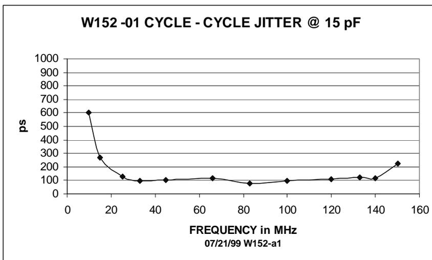
Figure 3. Cycle to Cycle Jitter at 15 pF
