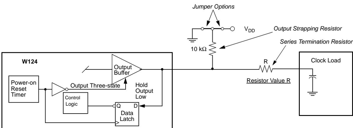
**Figure 2. Input Logic Selection Through Jumper Option**
